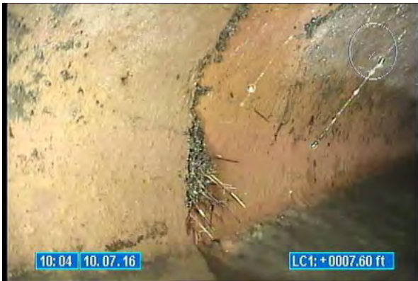
3520_ce242b34-08bc-4109-a9e0-498dbbd87258.jpg, 00:00:03, 7.60 Roots Fine Joint, from 07 to 10 o'clock, within 8 inch
