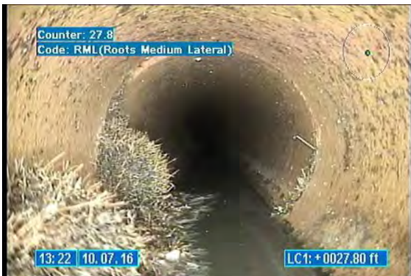
3410_0376d592-332a-4ce7-a68b-881beccd956d.jpg, 00:00:08, 27.80 Roots Medium Lateral, at 08 o'clock
