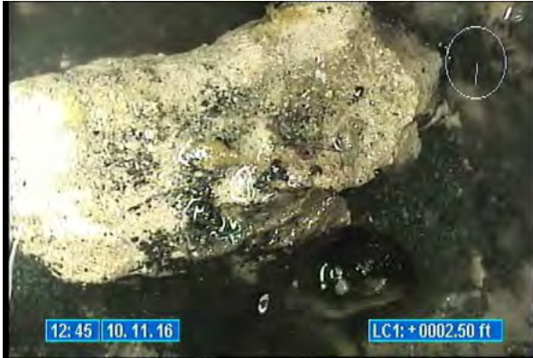
3620_69edcade-d517-4010-ab58-988f5f483955.jpg, 00:00:03, 2.50 Deposits Settled Other, at 06 o'clock
