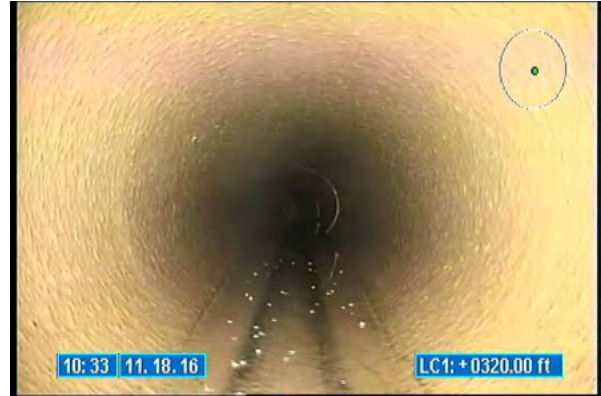
3350_8d179a1e-b423-4423-b50b-e80a0c9f58f9.jpg, 00:00:29, 320.00 Water Level, Sag in pipe, F02
